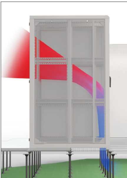
Cold air is directed to the cold zone by a deflector. A cold zone is created by an air separation frame, blank panels and a solid front door. The hot air leaves rack through a super-vented door.
