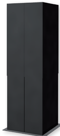
The chimney is designed to form a duct for the hot exhaust between the rack and the hot plenum. Its height can be adjusted from 750 mm to 1360 mm.
